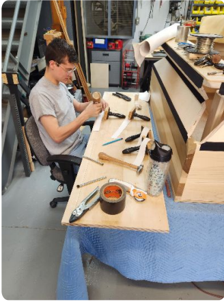
Zimmer team member Will repacks Bourdon pipe stoppers with leather to ensure a tight seal in the air passageway in the pipe.
