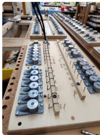
This close up of a bottom board shows magnets. Each pipe has a magnet and when a key on the console is pressed, the magnet opens a hole for the air to move through and allows the pipe to make sound.
