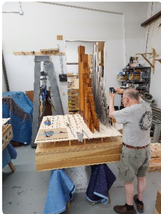
Jim, Zimmer's resident "pipe whisperer," fits each individual pipe to its hole in the windchest where it will live. Each of the 2,791 pipes in our organ is custom fitted to its windchest home.
