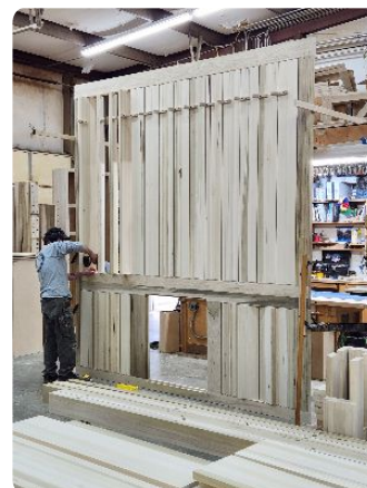
One of two expression shades which control the loudness and softness of sound from the pipes in the chambers.
