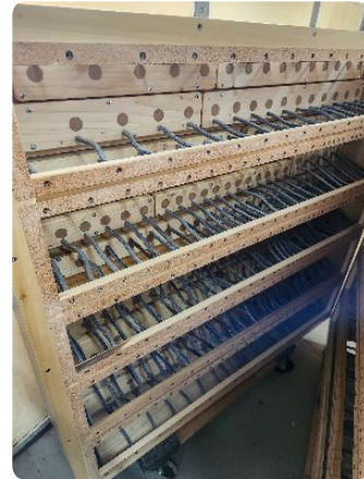
Pouchboards with rubber tuning connected inside the windchest.
