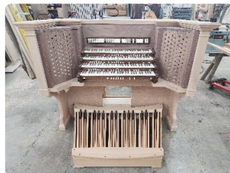
The console with keyboards and pedals. The next step is to dismantle the console and send the pieces to the paint chamber for staining and finishing. The outside and bottom of console are oak and will be stained to match the oak in the Sanctuary. The
