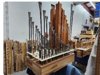
Jim fits the 16' English horn pipes to the windchest. These pipes have an interesting "funnel" shaped top to create the horn sound.
