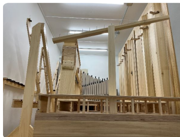
A view from the inside front of the Choir Chamber. The expression shades can be seen on the right, and the Bourdon pipes in the back.
