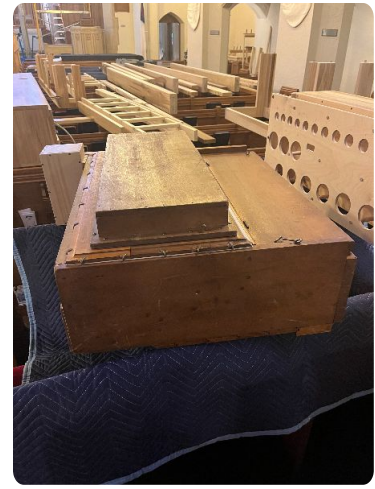
This is the vox humana, which has become part of our new instrument from a vintage 1930's organ at St. Peter's Episcopal Church in Charlotte, NC. A set of small reed pipes are enclosed in the wood box and the sound resembles the human voice.
