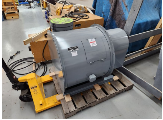
The blower motor, which will live in the newly renovated basement room.
