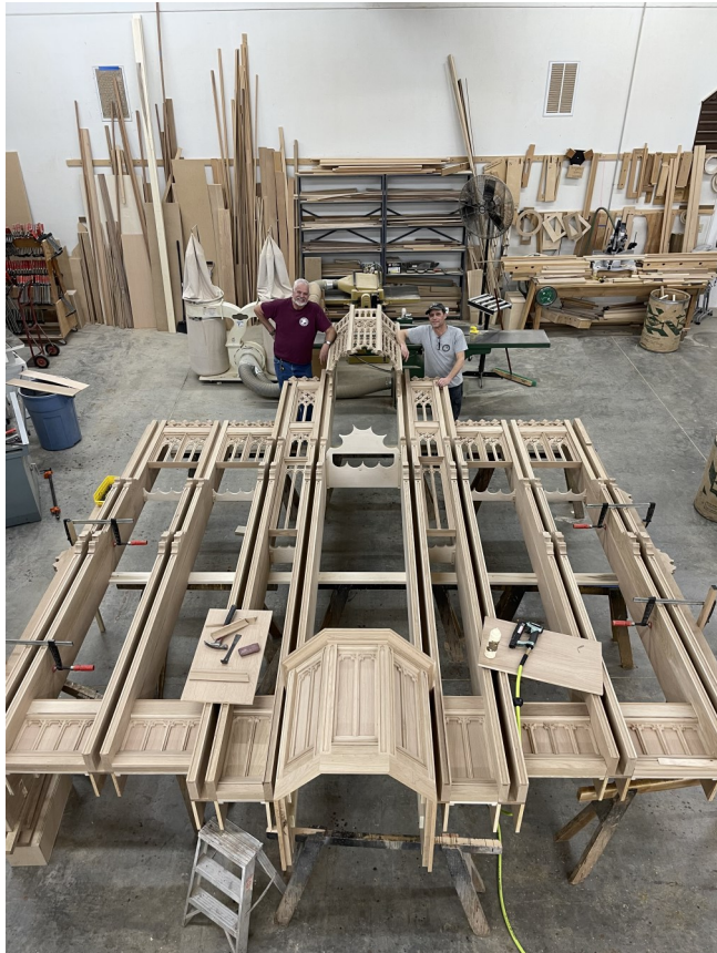
One side of the chancel casework, ready for staining and finishing.
