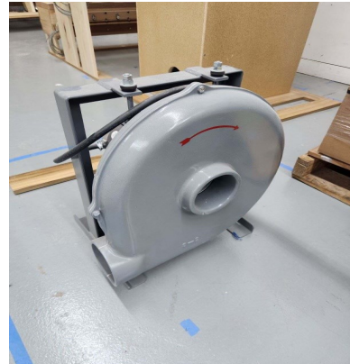
The blower fan, which will push air into the wind lines to allow the pipes to make sound. Located in the basement blower room.
