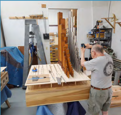
Jim Twyne, Zimmer Organ's voicer, fits pipes to their windchest in August 2023. (credit: CZOB)
