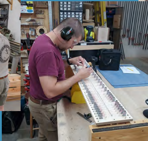
Zimmer technician Casey Snyder wiring magnets on a bottom board (credit: CZOB)
